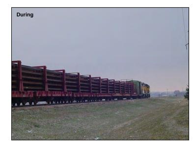
The D & I hauling with a load of 7 ½ miles of CWR at Elk Point, SD
