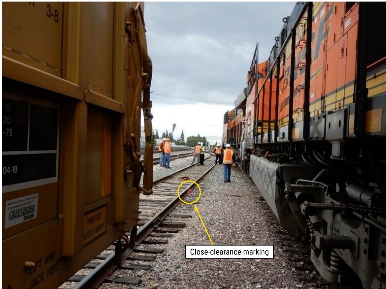
Figure 2. A marked close-clearance area in the La Mirada, California, accident investigation.
