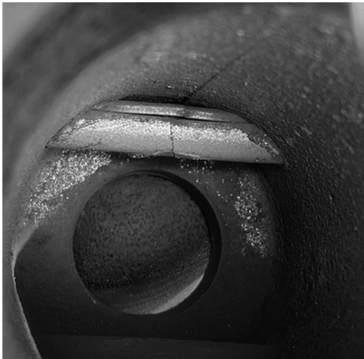
Figure 7-Roll pin crack on king pin
