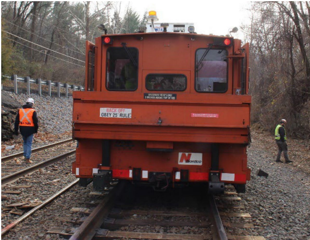
Figure 3. Standoff warning sign on the rear of Spiker 2.
